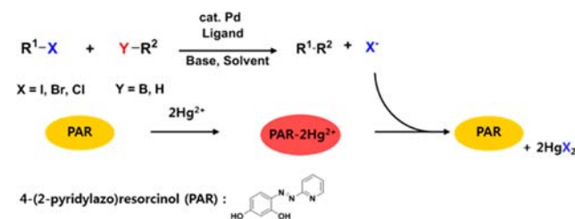
Scheme 1. Schematic Representation of the Halide Probe Based on a High-Throughput Screening Method for the Coupling Reaction of Aryl Halides
